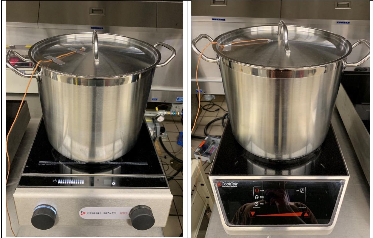
Figure 2: Water Boil Test for Induction Cooktops
