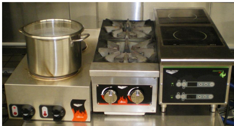
Figure 1: Commercial Cooktop Appliances (left to right): Electric Resistance , Natural Gas and Electric Induction
