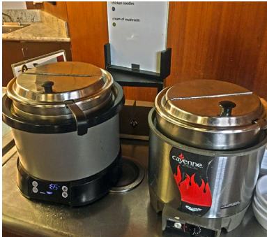
Replacement Induction Dry-Well Soup Warmer (left) and Baseline Wet-Well Soup Warmer (right)
